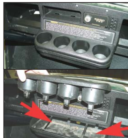
Fig 2 - EZ-GO Cup Holder Removal
