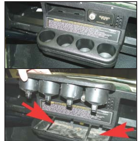
Fig 2 - EZ-GO Cup Holder Removal
